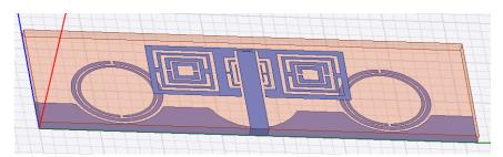
Fig. 6 Multiband antenna prototype using SRR and CSRR Simulated in HFSS
