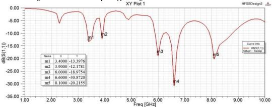
**Fig.7.** S11 verses frequency response for antenna
