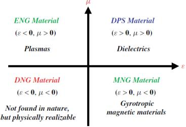
**Fig. 1.** Metamaterial classification based on  $\varepsilon - \mu$  [1]
