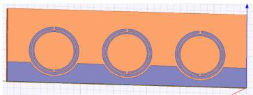
Fig.8. modified ground structure of antenna
