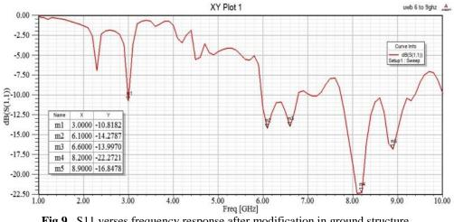
**Fig.9.** S11 verses frequency response after modification in ground structure.
