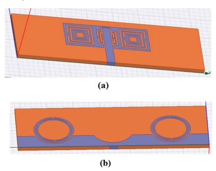
Fig.5. Multiband antenna using SRR and CSRR a) Top view b) Ground plane
